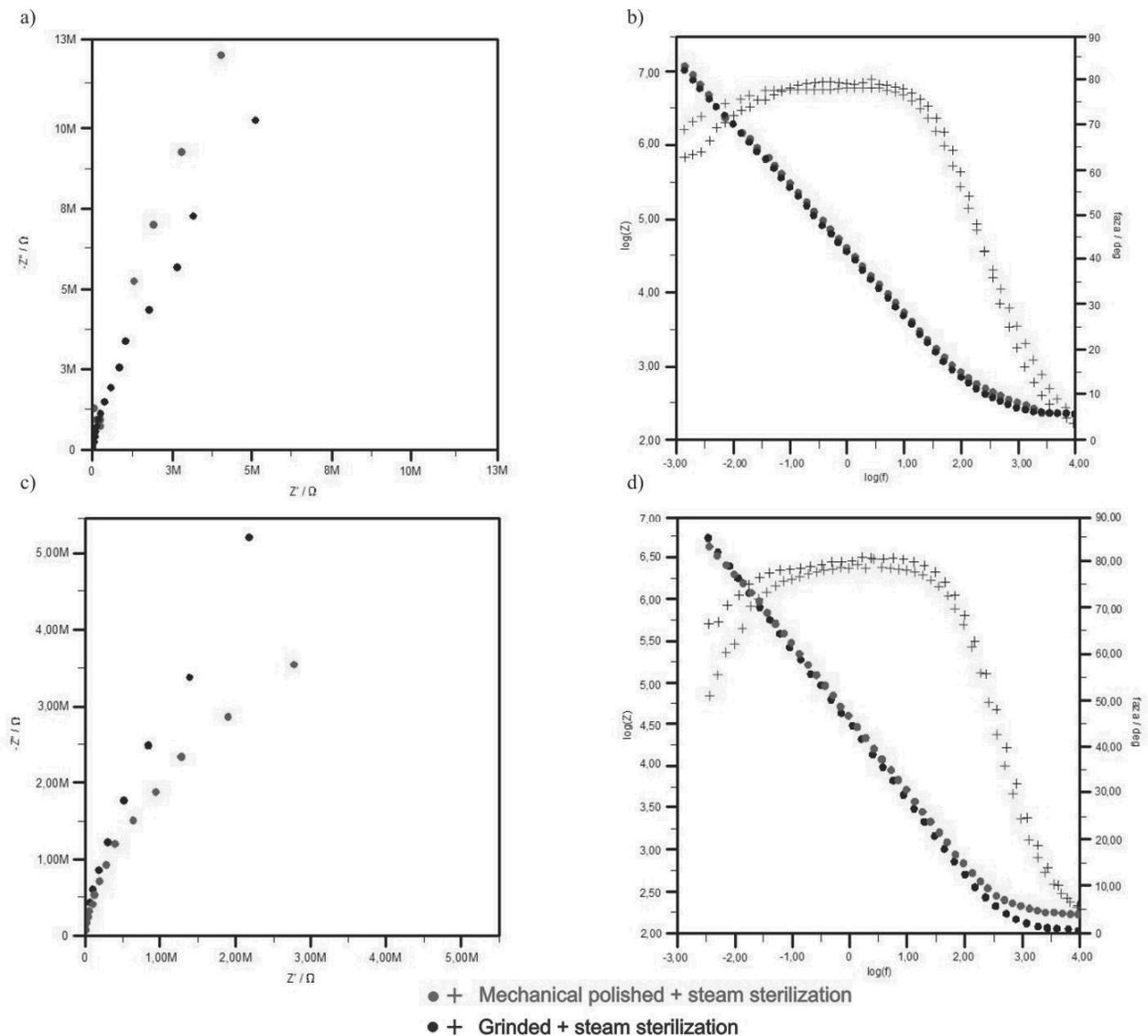
Fig. 9. Impedance spectrums for Ti-6Al-7Nb alloy test pieces: a) Nyquist diagram, b) Bode diagram, c) Nyquist diagram (after exposure in the Ringer's solution), d) Bode diagram (after exposure in the Ringer's solution)
