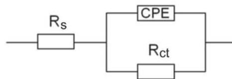
Fig. 6. Physical model for metal – passive film – solution system
