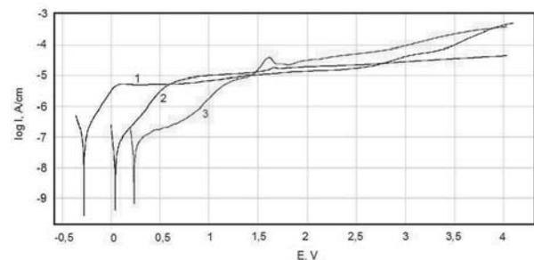
Fig. 2. Anodic polarization curves for Ti-6Al-4V alloy samples of surface: 1 – mechanically polished, 2 – mechanically polished and steam sterilized, 3 – mechanically polished, steam sterilized and exposed in Ringer's solution
