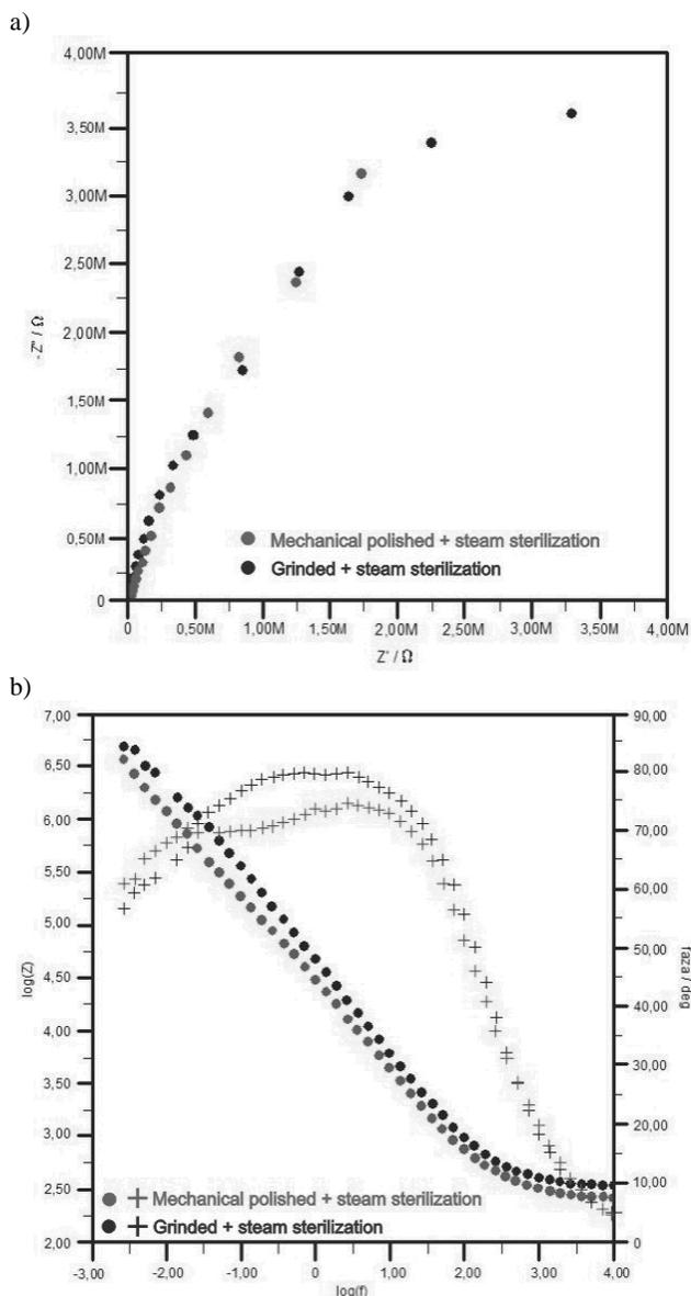
Fig. 5. Impedance spectrums for Ti-6Al-4V alloy: a) Nyquist diagram, b) Bode diagram
