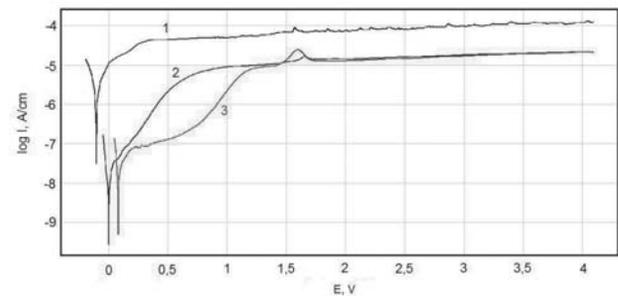
Fig. 4. Anodic polarization curves for Ti-6Al-7Nb alloy samples of surface: 1 – polished mechanically 2 –polished mechanically and steam sterilized, 3 –polished mechanically, steam sterilized and exposed in Ringer’s solution
