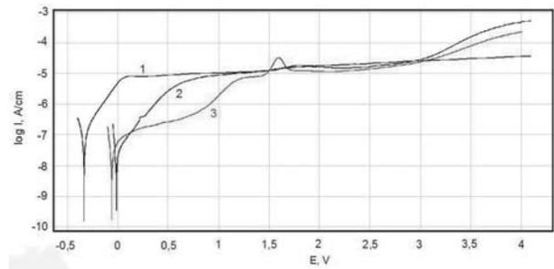
Fig. 1. Anodic polarization curves for Ti-6Al-4V alloy samples of surface: 1 – grinded, 2 – grinded and steam sterilized, 3 – grinded and steam sterilized and exposed in Ringer's solution
