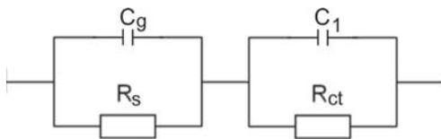
Fig. 8. Physical models for metal – passive film – solution system
