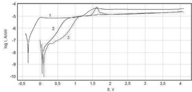
Fig. 3. Anodic polarization curves for Ti-6Al-7Nb alloy samples of surface: 1 – grinded, 2 – grinded and steam sterilized, 3 – grinded, steam sterilized and exposed in Ringer’s solution
