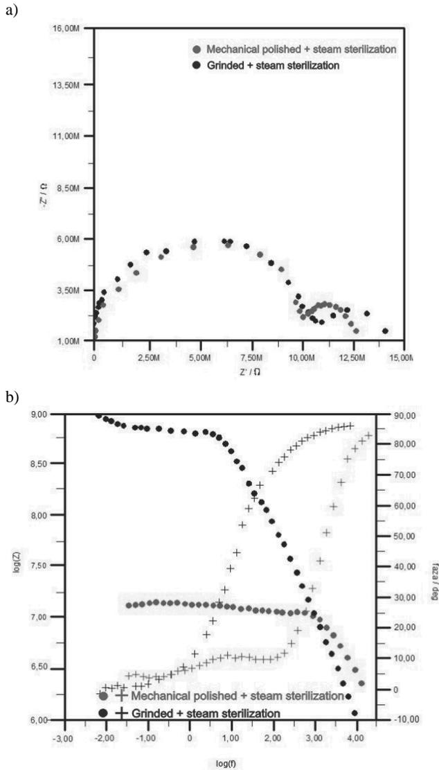
Fig. 7. Impedance spectrums for Ti-6Al-4V alloy after exposure in the Ringer’s solution: a) Nyquist diagram, b) Bode diagram
