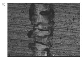
Fig. 7. a) Acoustic emission (AE) and friction force Ft as a function of the load Fn for the Ti(B,N) coating on sialon ceramics, b) the Scratch failure pictures of the Ti(B,N) coating on sialon ceramics at  $L_c$  (opt) = 13 N, mag. 200x
