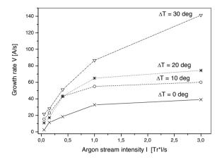
Fig. 11. Growth rate V dependence on technological conditions  $\Delta T$  and I
