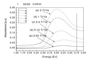
Fig. 3. UV-Vis spectra of PPI layers prepared with equal temperature of monomers,  $\Delta T = 0^{\circ}C$
