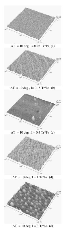
Fig. 8. Topographic images of series 2, prepared with  $\Delta T = \!\! 10$  °C and with increasing Ar stream intensity
