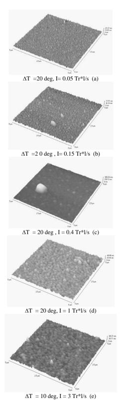
Fig. 9. Topographic images of series 3, prepared with  $\Delta T=20^{\circ}C$  and with increasing Ar stream intensity
