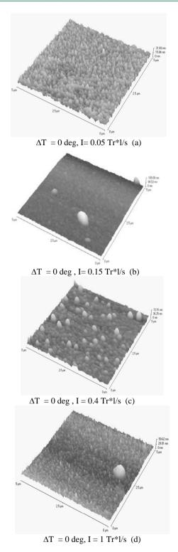
Fig. 7. Topographic images of series 1, prepared with  $\Delta T=0~^{\circ}C$  and with increasing Ar stream intensity
