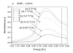
Fig. 5. UV-Vis spectra of PPI prepared with 10°C difference between monomer's temperature
