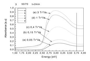
Fig. 4. UV-Vis spectra of layers prepared with 20  $^{\circ}\text{C}$  difference between monomer's temperature
