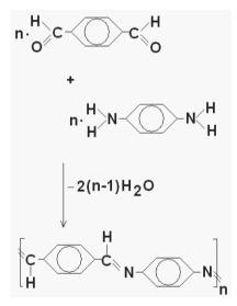
Fig. 2. Polycondensation of pol(1.4-phenylenemethylenenitrilo-1.4phenylenenitrilomethylene)
