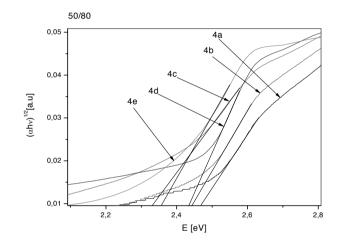
Fig. 15. Energy gaps E<sub>σ</sub> of PPI thin films
