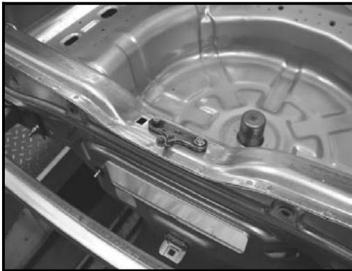
Fig. 3. The distance plate of the posterior boot door for the measurements of margins and external profiles
