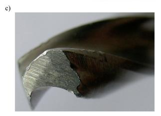
Fig. 5. Cutting edge of surgical drills: a - an initial state, b - cutting edge of the  $1^{st}$  drill after the wear tests, c - cutting edge of the  $2^{nd}$  drill after the wear tests
