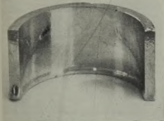
FIG. 1.—MACHINED CAST-IRON BEARING SHELL TINNED BY THE NEW PROCESS.
