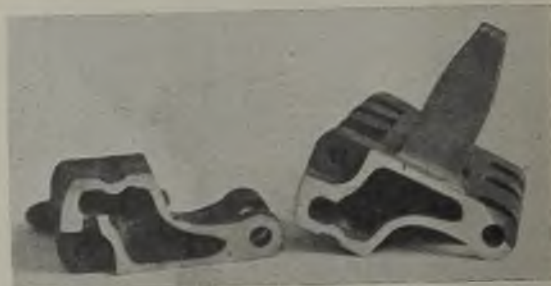
FIG. 6.—SECTIONED TRACK LINK SHOWING WALL THICKNESSES.
