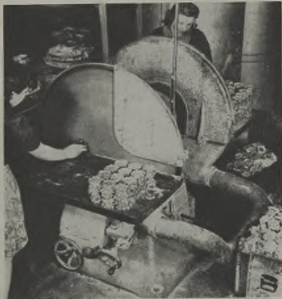
FIG. 45.—“CYLINDER BLOCK COVERS” BEING TRIMMED ON “WADKIN’S” DOUBLE-DISC GRINDING MACHINE.
