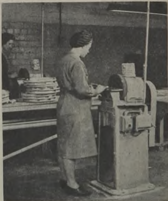
FIG. 42.—TRIMMING OF "UNDERCARRIAGE PUMP DRIVE COVERS" BY "RINDIS" RING AND DISC FILING MACHINES.
