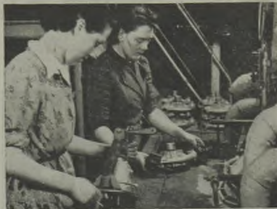
FIG. 48.—PRESSURE TEST—CLAMPING JIGS TO CASTING.
