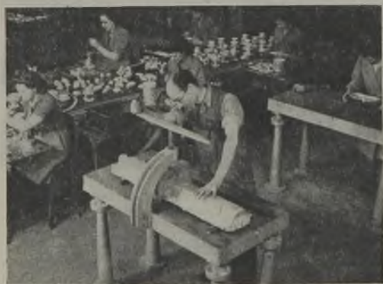
FIG. 51.—STRAIGHTENING OF "ROCKER COVER" BY SCREW PRESS.
