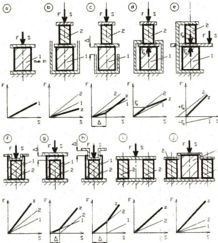
Fig.2. Relation R in an assembly consisting of two different elements and their influence on the curve of characteristics
