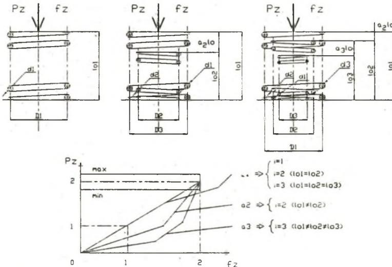
Fig.5. Construction variant and the possible changes in the  $Pz$  loading of an assembly in relation to the deflection  $fz$
