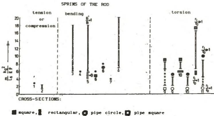
Fig.3. Comparison of springs for the  $m/L_s$  criterion according to R. Herber [5] (Notation for types of springs: 1 - rod; 2 - ring; 3 - flat rectangular; 4 - flat triangular; 5 - flat trapezoid; 6 - spiral; 7 - helical torsional; 8 - disc; 9 - torque rods; 10 - helical cylindrical tension; 11 - helical conical telescopic)
