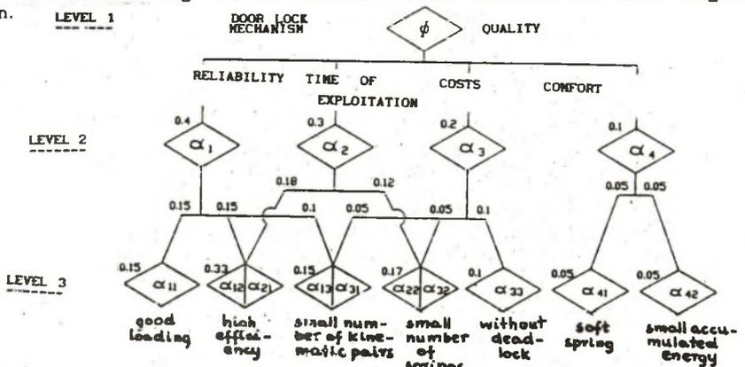
Fig. 4. Criteria and weights during selection of the mechanism
