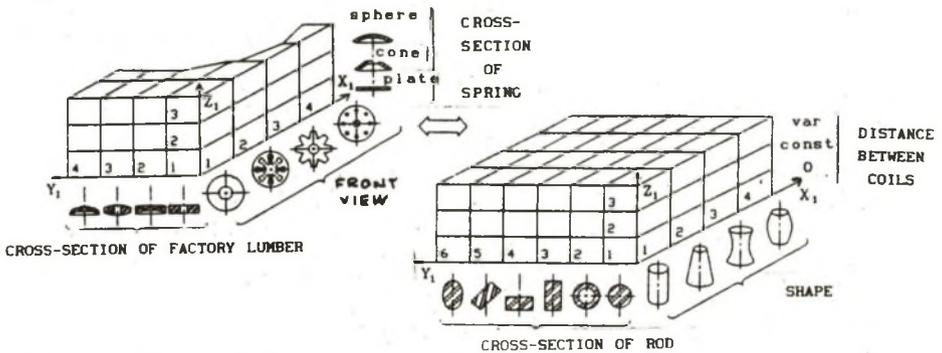
Fig.1. Form of construction of E elements (disc and helical spring class)
