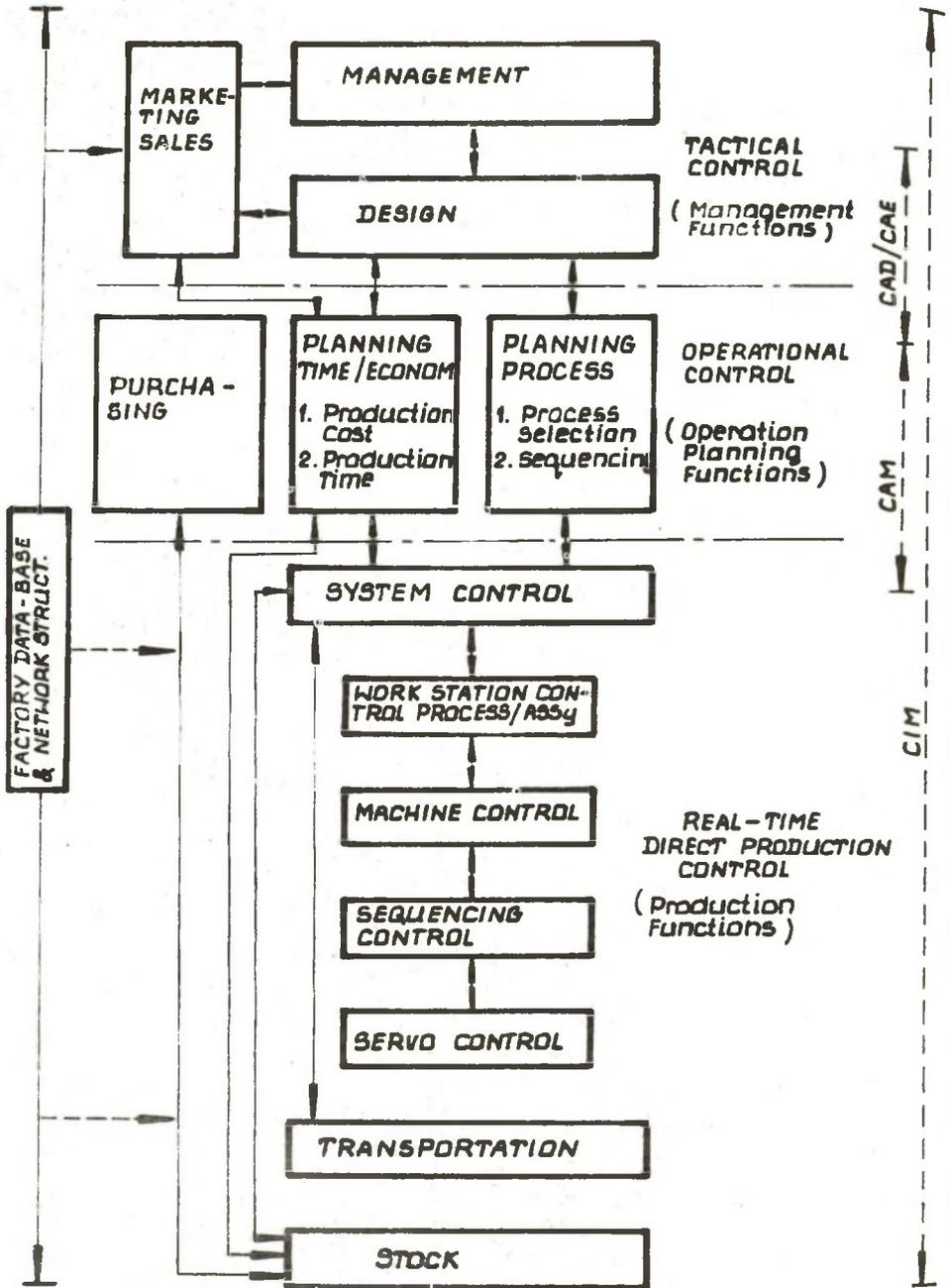
Fig. 1 Reference Model of Manufacturing Control System
