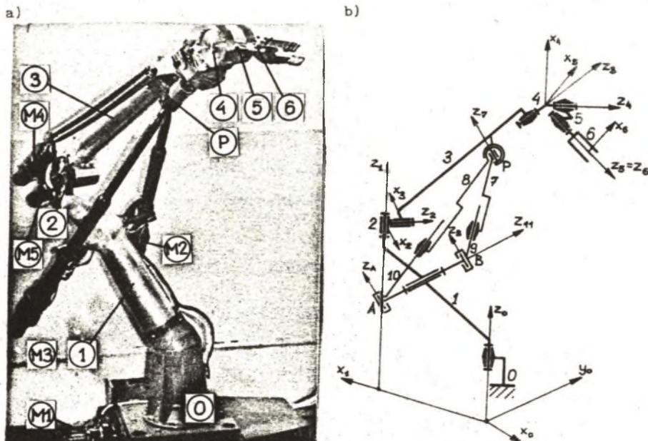
Fig. 1. Manipulator of serial-parallel structure: a) prototype, b) scheme
