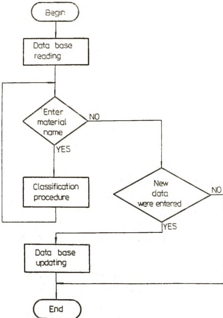
Fig. 2. Algorithm of the classification program
