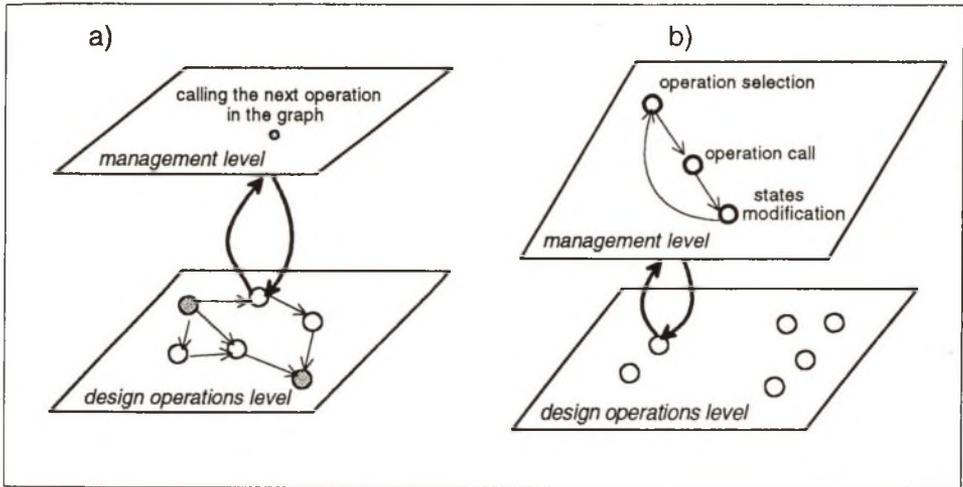
Fig. 1. CAD systems organization: a) of a fixed course of task solving, b) of an undetermined course of task solving
