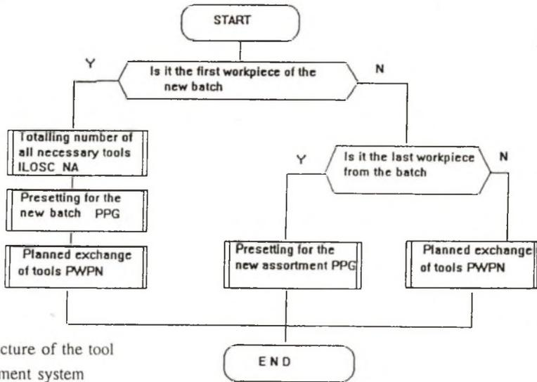
Fig.3. The structure of the tool management system
