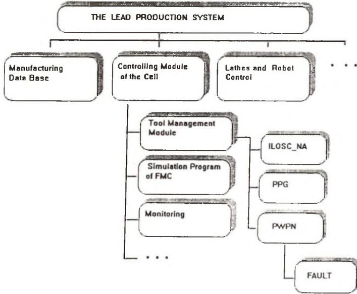
Fig.1. The tool management system as one of the modules the cell control system.
