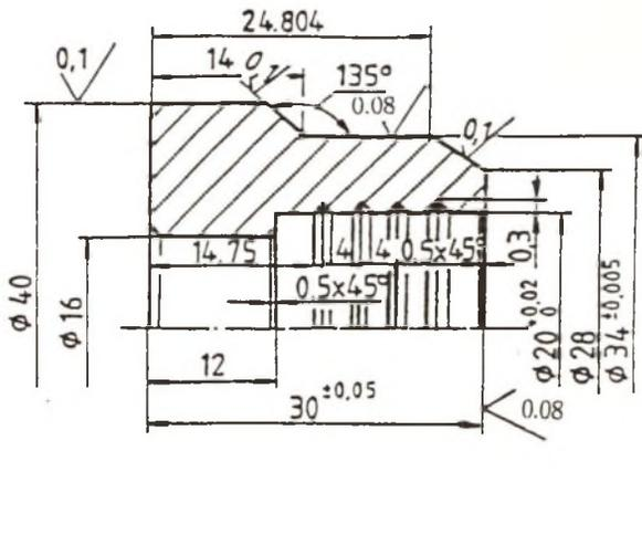
Fig.3. Part made of hardened steel
