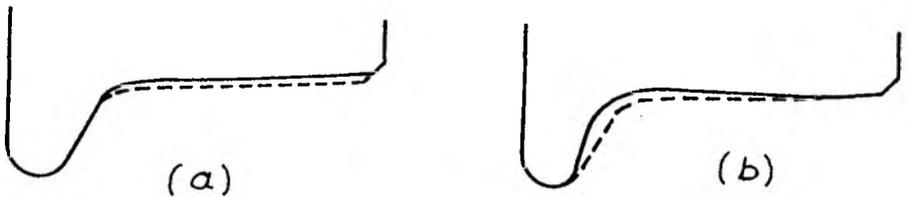
Fig. 2. Wheel wear patterns for (a) predominantly tangent track running, and (b) predominantly curved track running
