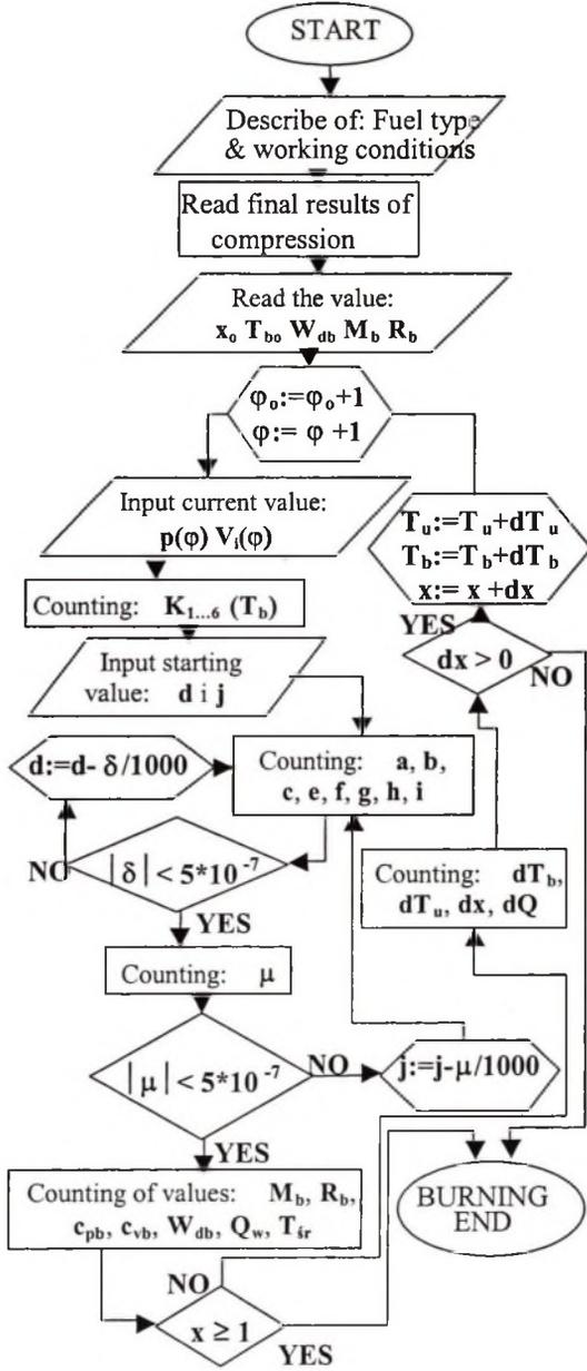
Fig. 2. Algorithm of solving dual-zone model of combustion
