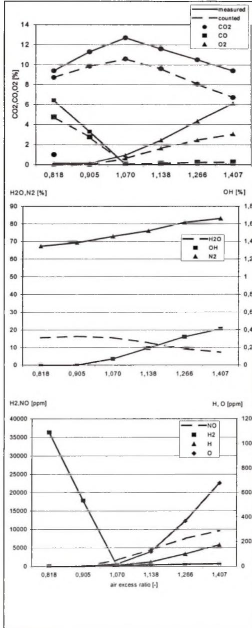
Fig. 6. Exhaust gases composition in dependence on air excess ratio, for throttle opening ratio 50%, rpm 1750, ignition advance 12°
