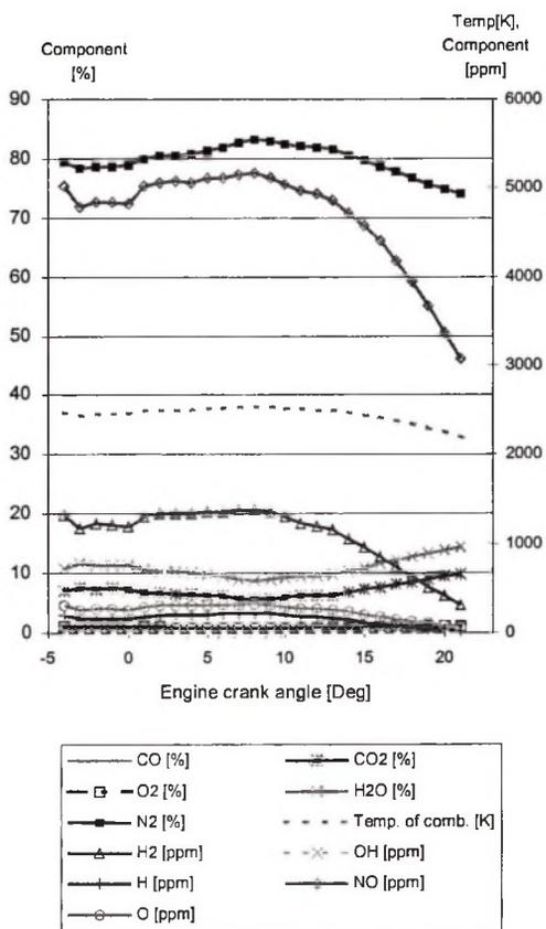
Fig. 5. An example of forming 10 components of exhaust gases during combustion, throttle opening ratio=50%, rpm 1750, air excess ratio 1,08 and ignition advance  $5^{\circ}$
