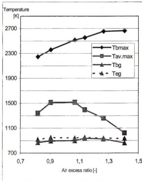
Fig. 3. Characteristic temperatures of combustion in dependence of air excess ratio. Throttle opening ratio=25%
