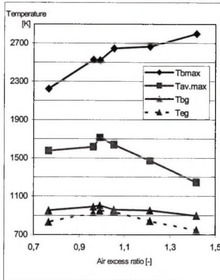
Fig. 4. Characteristic temperatures of combustion in dependence of air excess ratio. Throttle opening ratio=50%
