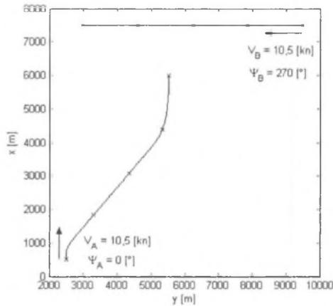
Fig.3. Trajectories of ships in an encounter situation in an open area; simulation time 1200 [s]; positions (x) at 300 [s] time intervals;
