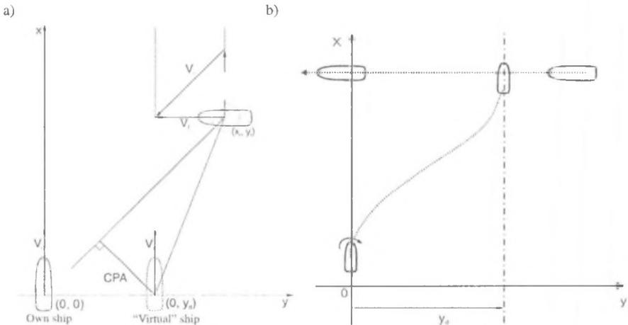
Fig.2. The method for determining a safe trajectory using a 'virtual' ship: a) virtual ship's position; b) parallel trajectory
