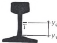
Fig.5. Arrangement of the coil concerning a rail
