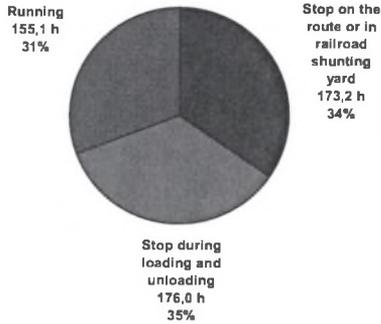
Fig.1. Breakdown of runs and stops of a typical example of cross-border rail freight traffic [1]
