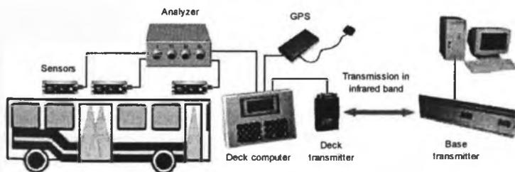
Fig.2. Concept diagram of the IRMA system (source: website of Emтал Sp. z o.o.: <http://www.emtal.pl>)
