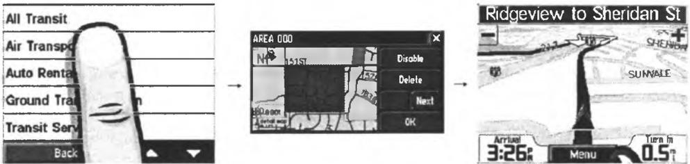
Fig.4. Road route planning, taking criteria (i.e. an area to be avoided) into account [6]
