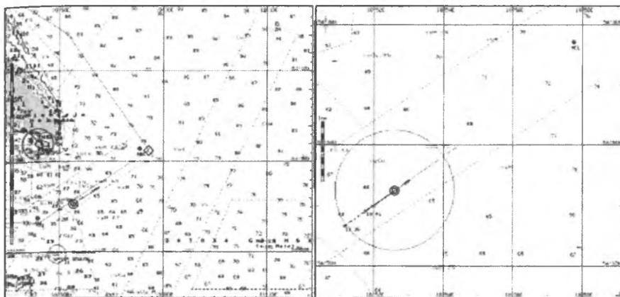
Fig.5. Following a passage plan (left), and monitoring of: *dangerous area* and *dangerous depth* limits (right), by means of a maritime electronic chart system
