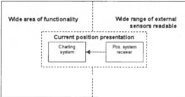
Fig.3. Positioning as a core of electronic charting system
