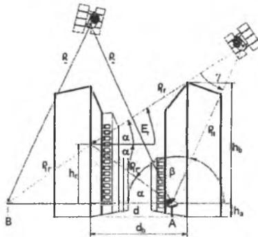
Fig.6. Error of position caused by satellite signals reflection [3]
