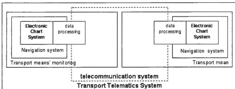
Fig.1. Location of electronic chart systems in the Transport Telematics System [4]
