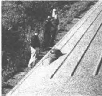
Fig.8. Installation of the IAT-Terminal in a newly designed PESA-sleeping car (PKP), the antenna is visible on the roof of the vehicle [5]
