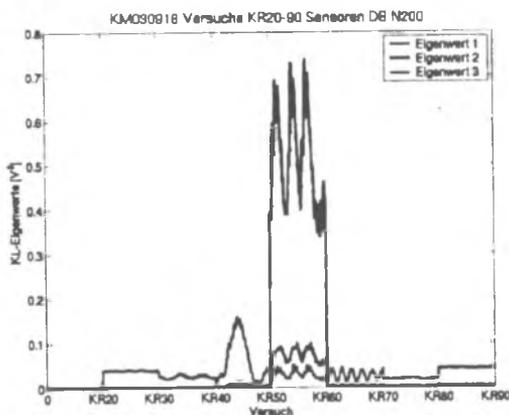
Fig.6. Analysis of a wheel set rolling trial by KL-transform ( $1 \text{ V}^2$  equals  $100 \text{ g}^2$ )
