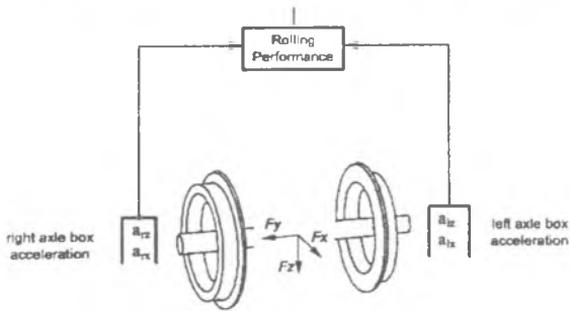
Fig.5. Prinziple of determination of wheel set rolling performance
