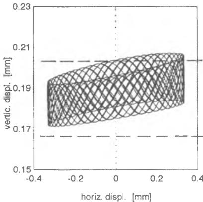
Fig.3. Simulation of the axle bearing orbits of an ICE wheel set, which undertakes bending/torsion vibrations due to static and dynamic out-of-balance (SZOLC 1995)
