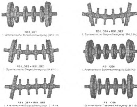
Fig.2. Medium frequency eigen-dynamics of an unbounded ICE wheel set [2]
