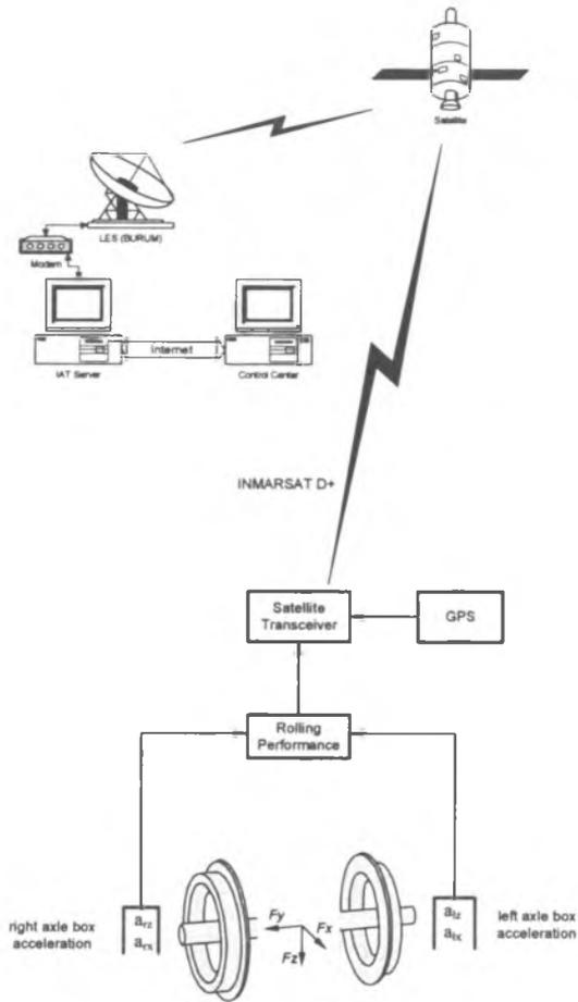
Fig. 9. Event monitoring of the rolling performance of wheelsets
