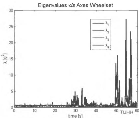
Fig.7. Rolling quality of an ICE wheel set, running on a bad conditioned track section
