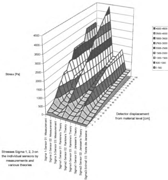
Fig.9. A 3D graph of the mutually dependent normal stresses of BraLEN recorded on a 3D indicator in the silo (Fig.6) and how they stand up to the theories. Source: [9]
