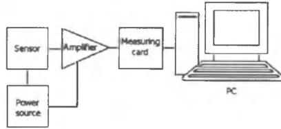
Fig.1. A description of the measuring system consisting of the power source, tensometric sensor, measuring amplifier, measuring card NI and PC. Source: [9]
