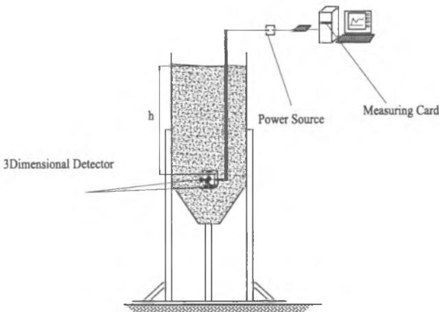
Fig.5. The setup of the 3Dimension indicator – the power source-terminal box-measuring card and the indicator for measuring pressure in the storage equipment. Source: [9]
