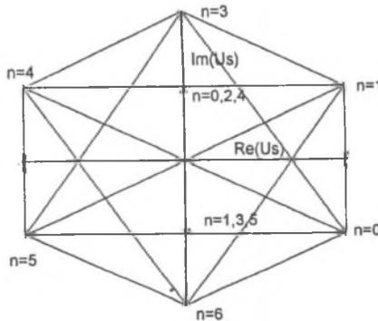
Fig. 3. Symmetrical voltage vectors for B4 configuration
