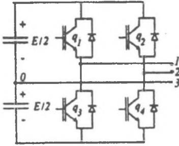
Fig. 1. Three-phase drive using B4 inverter
