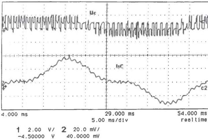
Fig.5. Experimental results: phase C voltage and steady-state stator current in B4 configuration
