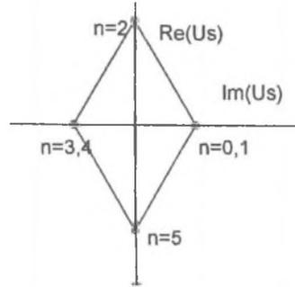
Fig. 2. Voltage vectors in B4 configuration
