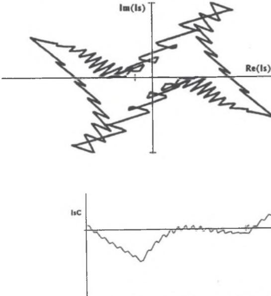
Fig.4. Stator steady-state current trajectory and phase C current
