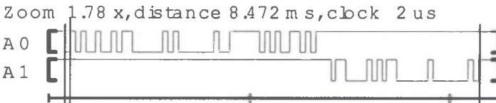
Fig. 6a: Time between start and end communication for speed 9600 bauds
