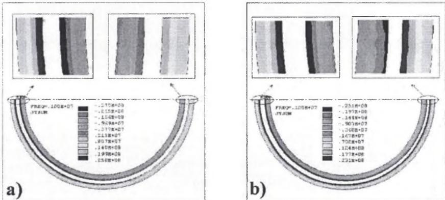
Fig. 9. The distribution of the current in the windings of (a) BT and (b) NCT arrangement
