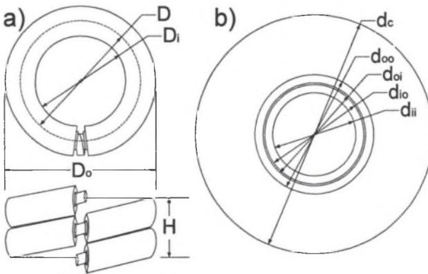
Fig. 2. Dimensions of the basic transformer (BT): a) top and front view; b) cross section of the windings and magnetic core
