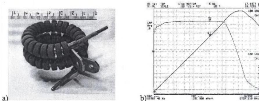
Fig. 10. The prototype transformer (a) and its  $|Z|$  and  $\theta$  characteristics vs frequency (b)
