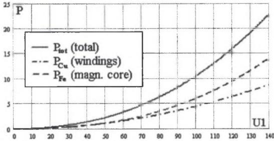
Fig. 4. The power losses in the basic transformer (BT) versus input voltage (rms value)
