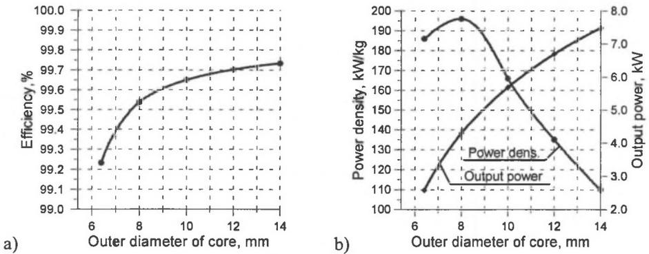
Fig. 6. The efficiency (a) and power (b) of the transformer vs outer diam.  $d_c$  of magnetic core
