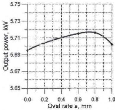
Fig. 8. Output power versus oval rate in OCT transformer
