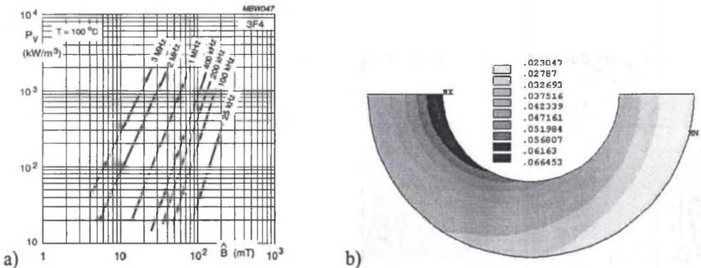
Fig. 3. The specific power losses (a) and distribution of flux density (b) in the magnetic core
