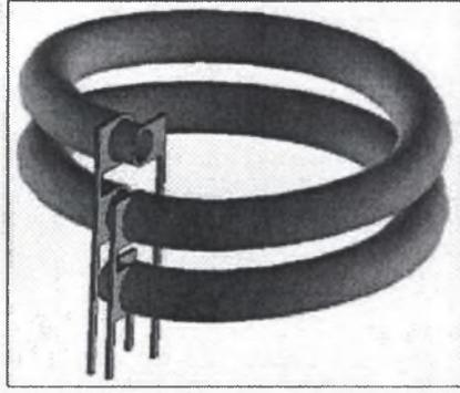
Fig. 1. Windings of the basic transformer (BT) (without magnetic core)
