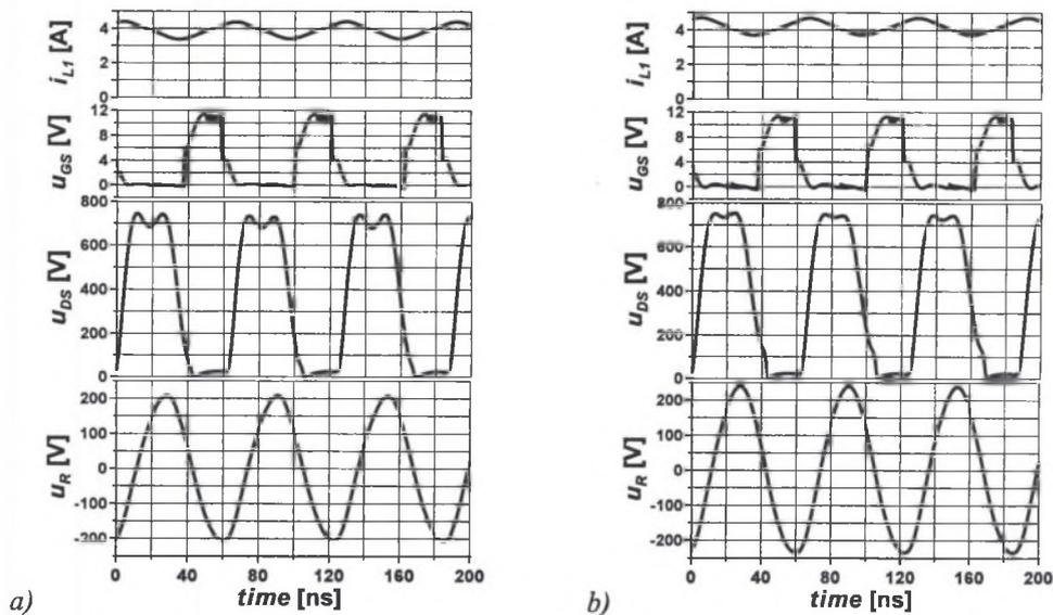
Fig. 10. Simulated waveforms of Class EF SPICE model for load resistor 16,5  $\Omega$  (a), 20  $\Omega$  (b)
