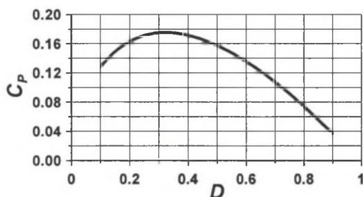
Fig. 8. Power output capability vs. switch "on" duty ratio of Class E inverter
