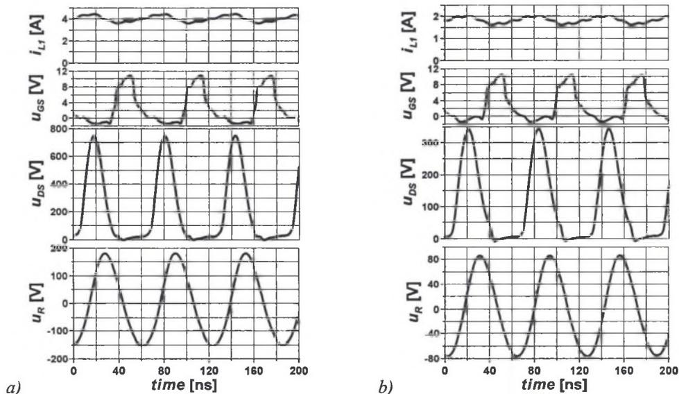
Fig. 5. Measured waveforms of currents and voltages for supply voltage  $E=220$  V (a), and 110 V (b) ( $i_{L1}$  - supply current,  $u_{GS}$  - gate-source voltage,  $u_{DS}$  - drain-source voltage,  $u_R$  - load voltage - fig. 2)
