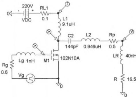
Fig. 6. Class E SPICE model, 800 W, 16 MHz
