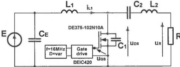
Fig. 2. Class E inverter schematic
