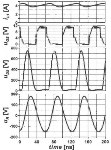
Fig. 7. Simulated waveforms of Class E SPICE model
