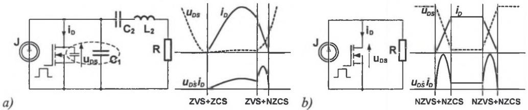
Fig. 1. Class E operation (a) vs. hard-switching (b)
