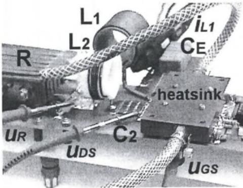
Fig. 3. Main components of laboratory inverter
