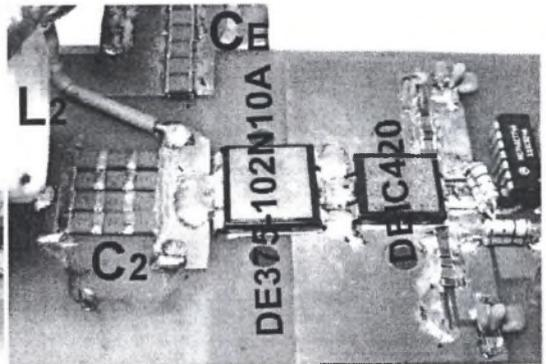
Fig. 4. DE375-102N10A MOSFET transistor and DEIC420 gate driver
