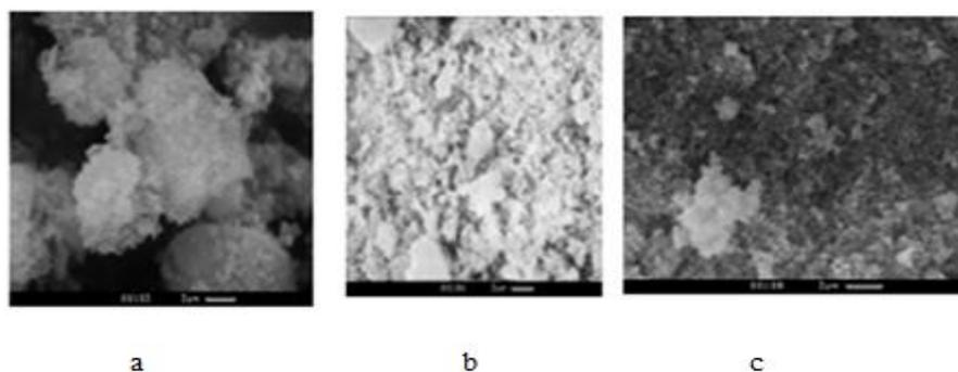
Fig. 1. SEM – images of plate-like sorbent surfaces, obtained from calcium silicate powders by standard synthesis (a), with PVA addition (b), by microemulsion method with quaternary ammonium base (c)
