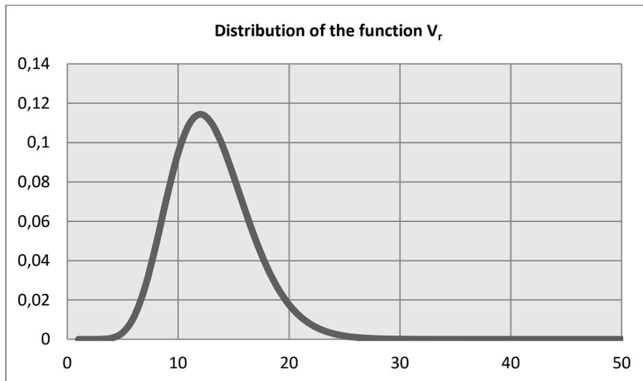
Fig. 3. Distribution of the function describing the shearer working speed  $V_r$
