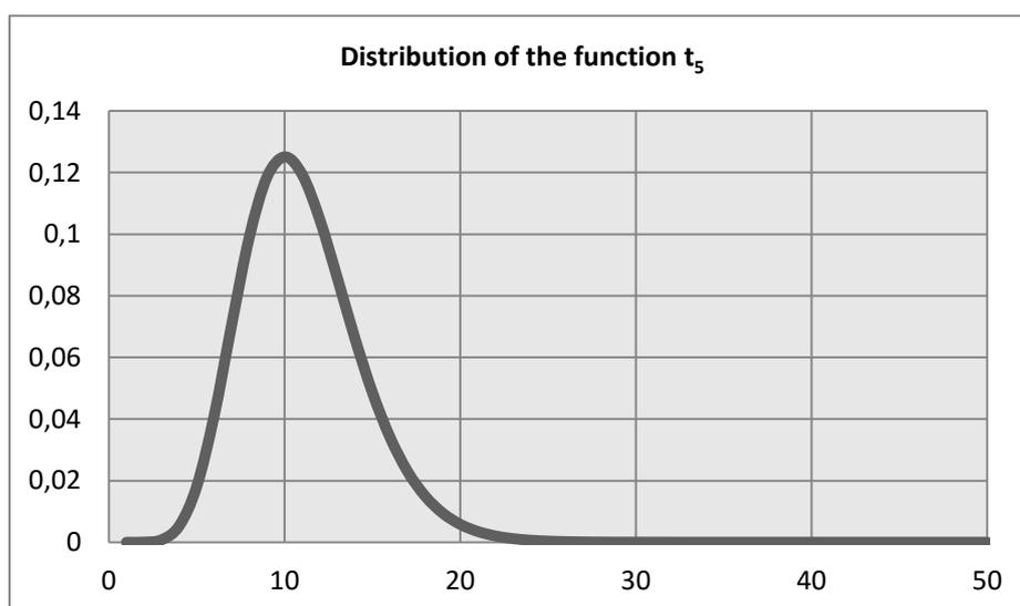
Fig. 6. Distribution of the function describing the drive movement time  $t_5$
