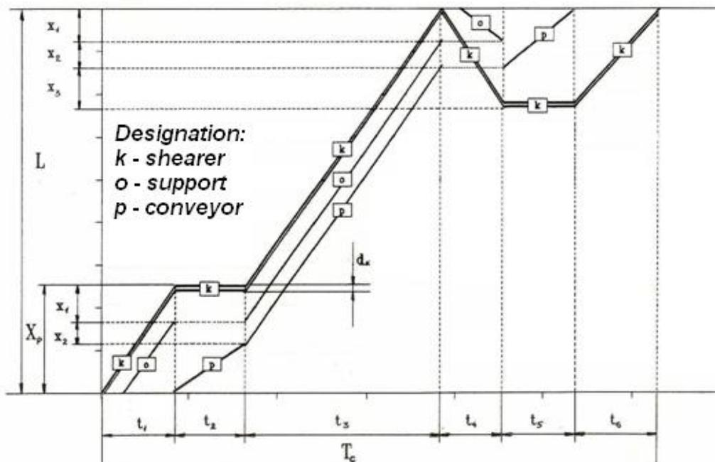
Fig. 1. Diagram of the production cycle for the bidirectional shearer cutting technology
