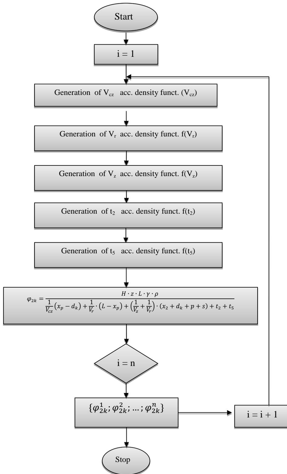
Fig. 7. Calculation scheme for the output stream rate index in the bidirectional shearer cutting technology
