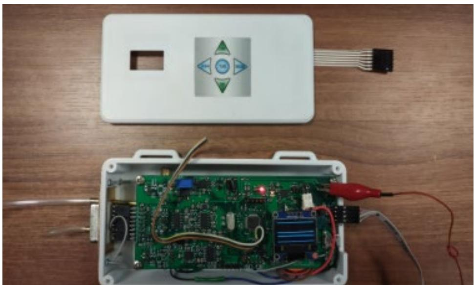
Fig. 5. Assembled unit with 3D printed case
