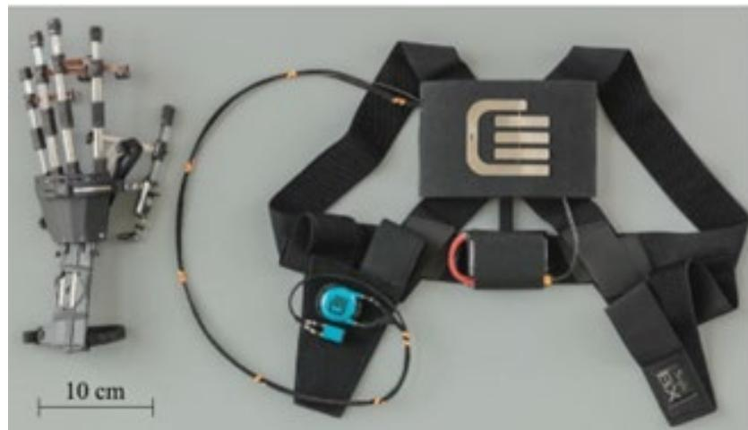
Fig. 12. Exoskeleton RELab tenoexo [21]
