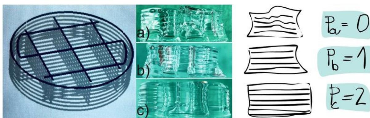
Fig. 4. Printability evaluation of printouts, Side view
