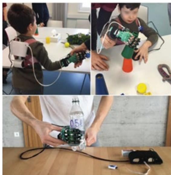
Fig. 13. Grip therapy with physical exercises using the PEXO exoskeleton [21]
