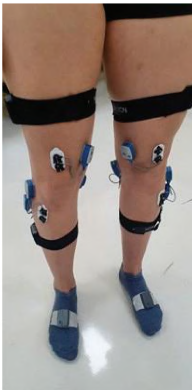
Fig. 2. Arrangement of EMG electrodes
