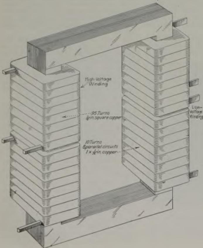
water service lines in some of the company's houses. With this transformer, our men have thawed out pipes in twenty different houses in less than five hours. To facilitate the work the transformer was hauled around on a truck and connected to a large lighting transformer.
