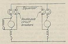
Fig. 3-Two-Pole Breakers Prevent All Flashing
