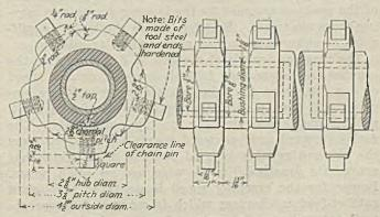
Fig. 1—Details of the Digging Sprocket
