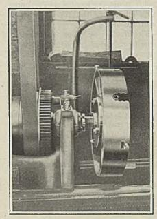
Screwing Chuck Onto Spindle
