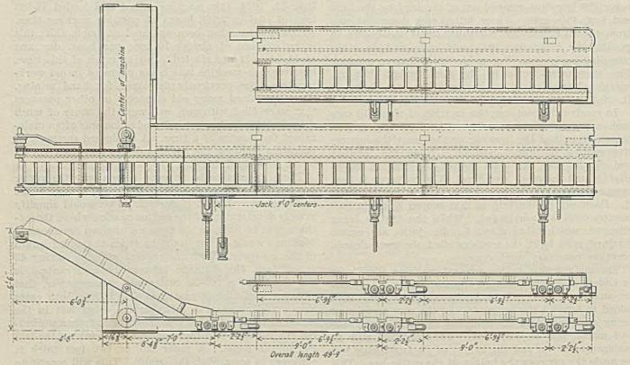
Plan and Side Elevation of the Machine
