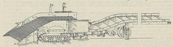
Stockly Machine Operates on Caterpillars Forcing Chain Conveyor with Digging Bits Under Coal—Overall Height Is 28-In.—It Is Adaptable to Car or Conveyor Loading
