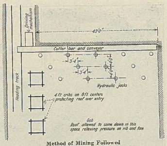
Advance is fairly steady and the only timber used is that necessary for building cribs. Behind the jacks the roof is allowed to come down freely into the gob. When the machine has advanced to the end of the heading it may be turned around so as to return either taking a cut from the opposite rib of the same heading or it can be brought back in the next parallel heading to the right.
