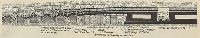
Fig. 9-Cribbing and Roof Action Behind a Face
