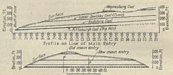
Profile on Line of 3rd Left Entry Extended, Showing also the Extent of First Mining on Big Vein
